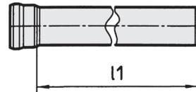
**GM-X drain pipes with two sockets 1 A in acc. to EN 1123 form B2**
