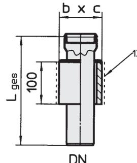
**GM-X Deck and bulkhead penetrations in accordance to DIN 86288**
