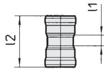
**Push-in sockets with long socket in acc. to EN 1123 form F5**
