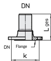
Vacuum installation in DN 40, DN 50, DN 70 with special GM-X-VACplus sealing element and standard x-socket piping system
