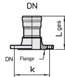
**GM-X spigot flange without mating flange form M2 in accordance to DIN 86288**
