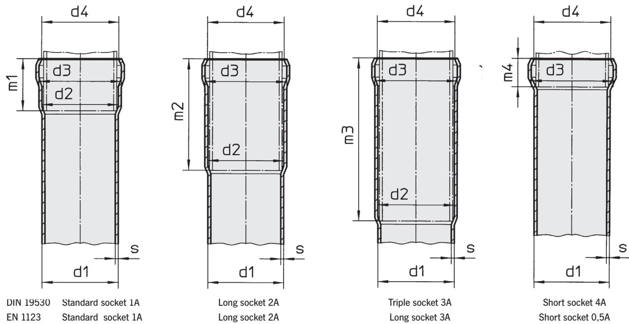
For pipes and fittings with 2 sockets both sockets are the same design
