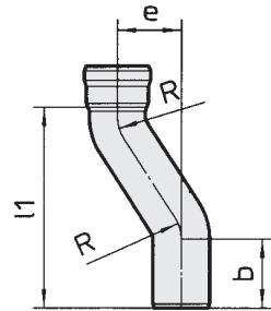
**Bends with calming section for transition into horizontal pipes**
