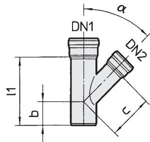
Vacuum installation in DN 40, DN 50, DN 70 with special GM-X-VACplus sealing element and standard x-socket piping system
