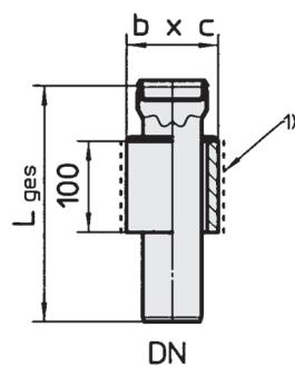
GM-VAC WC connector deck penetration in accordance to DIN 86288
