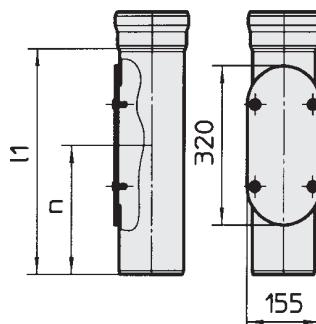
Clear width of cleaning aperture = 265 x 100 mm.
