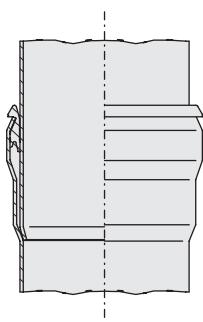
Socket DN 250 with set of seal
