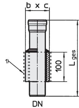
**GM-X Deck and bulkhead penetrations form R1A and R1B in accordance to DIN 86288**
