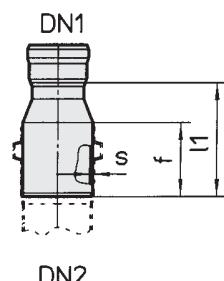
**Connectors for changing from GM-X pipe to plastic pipe socket as per
