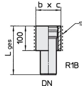
Vacuum installation in DN 40, DN 50, DN 70 with special GM-X-VACplus sealing element and standard x-socket piping system
