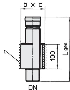
**GM-X Deck and bulkhead penetrations form R1S „Sanitary block“**
