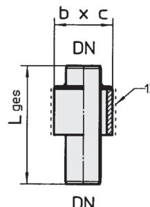
Vacuum installation in DN 40, DN 50, DN 70 with special GM-X-VACplus sealing element and standard x-socket piping system
