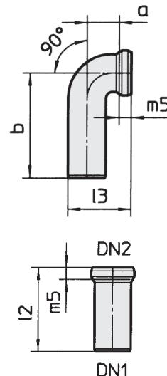
WC-connections, straight with inserted seal
