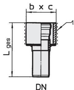
**GM-X Euro-WC deck penetration with sealing element**
