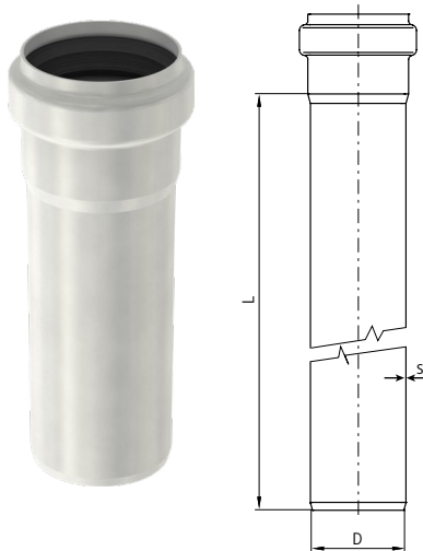
AP socketed pipe 40 mm according to EN-1124 form B1
