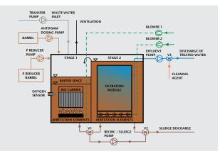
Biochemical phosphorus removal is achieved by dosing with aluminum or iron-based coagulants which ensure the effective precipitation of the phosphorous during the final filtration stage.
