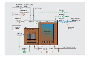
Biochemical phosphorus removal is achieved by dosing with aluminum or iron-based coagulants which ensure the effective precipitation of the phosphorous during the final filtration stage.
