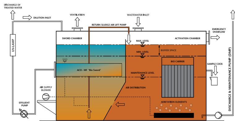
Clean water from the mixed liquor in the sword chamber is drawn through the ACO-MF 'bio-sword' by the effluent discharge pump (an optional standby unit is available) and discharged either directly overboard or alternatively to be recycled back into ship's storage for re-use as technical fresh water for all non-potable requirements such as toilet flushing, deck washing or even laundry applications.
