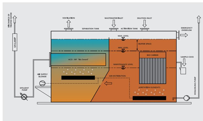
Clean water from the mixed liquor in the sword chamber is drawn through the ACO-MF 'bio-sword' by the effluent discharge pump (an optional standby unit is available) and discharged either directly overboard or alternatively to be recycled back into ship's storage for re-use as technical fresh water for all non-potable requirements such as toilet flushing, deck washing or even laundry applications.
