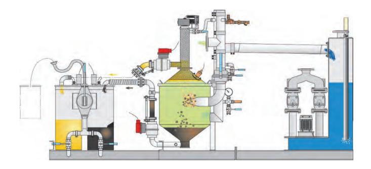
The shape of separators should be such to encourage efficient separation whilst at the same time having 'clean' internal surfaces that do not allow build-up of solids behind frames or in corners. The most effective design is a cylindrical concept with cones mounted top and bottom, like the system pictured. This affords more effective channelling of FOGs and solids to the discharge points.
