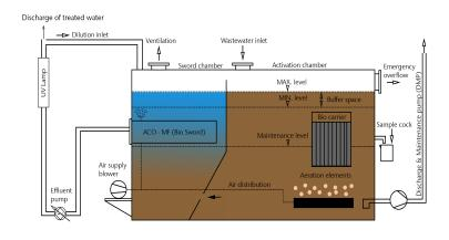
Disinfection of outlet treated water is carried out by the unit mounted UV lamp. A separate Discharge & Maintenance Pump (DMP) provides the higher capacity de-sludge and emptying requirement. Treated effluent water is colourless and odourless. Discharge is controlled by level control connected to the effluent discharge pump.
