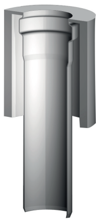
Penetration form R1B with a black pod with opened bottom, for direct welding in the deck | acc. to EN 1124 form T2 A0-A60
